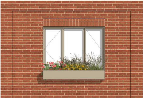
Elevation - Window Box Detail 1 : 25
